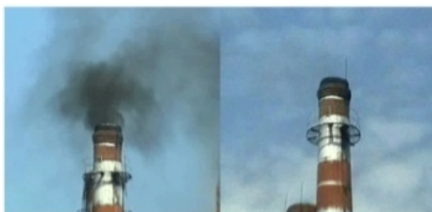
Fig. 17. Comparison of emissions in the process of combusting mazut and composite fuel
